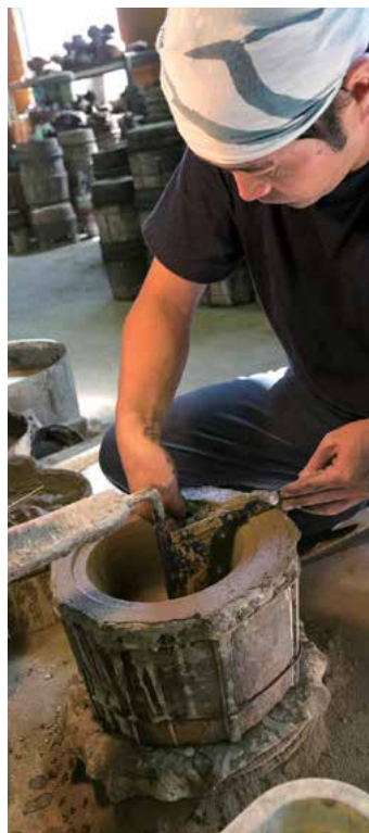
Left: Mixing clay with mud-like casting sand to create a mold for casting
